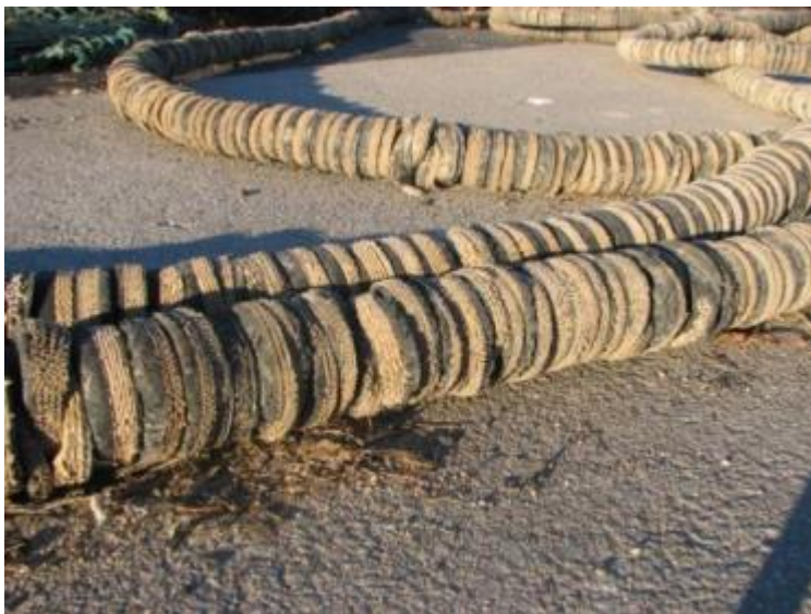
Figure 2 – Ground cable with cookies
